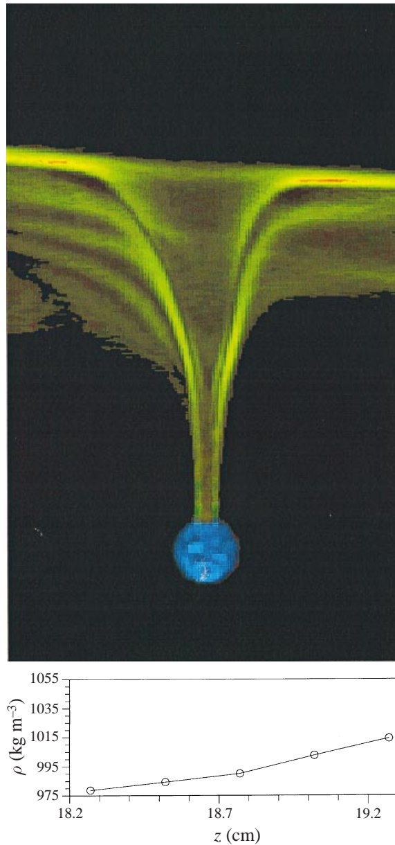
FIGURE 6. A particle passing through the interface and the density profile within the field of view. No morphological filtering was applied in this figure. d_p = 1.3 mm.
